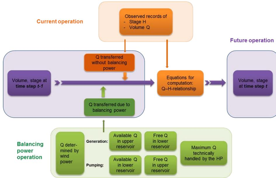
Fig. 1. Schematic model of how the future operation of hydropower plants with increased capacity was calculated
