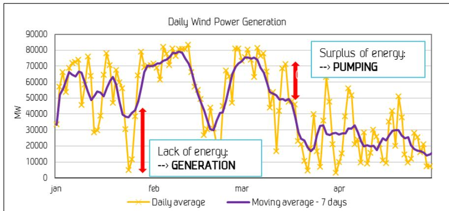
Fig. 2: Example of a period with both surplus and deficit of wind power that leads to pumping and production modes
