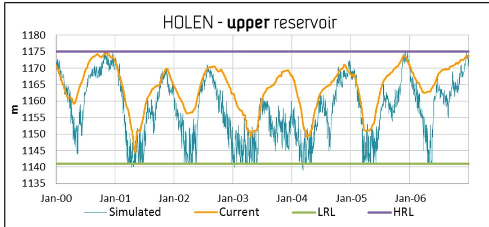
**Figure3. An example of water level variations in the upper reservoir for Holen power plant with current (observed) pattern (yellow) and simulated with balancing power with the 7Days-Avg scenarios for the years 2000-2006**
